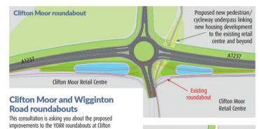
The blueprint for improving the capacity at all the roundabouts is based on providing three lane entries on the Ring Road approaches to the roundabout and two lane exits. This will provide an increase in the junction capacity similar to those implemented at the A59. A19 and Wetherby Road roundabouts.
